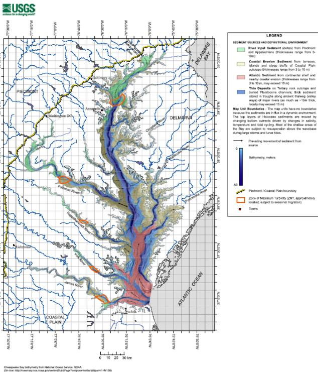
The USGS has mapped sediment sources near the Bay. This map delineates sediment from rivers, coastal erosion, and the Atlantic Ocean. Highlighted in red is the area of maximum turbidity (**Newell and others**). It is available online at: <http://pubs.usgs.gov/of/2004/1235/>
